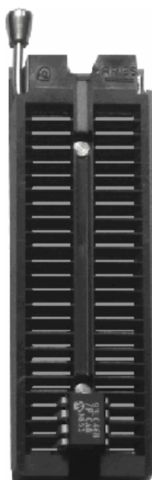
(a) Insertion of device 93LC46
